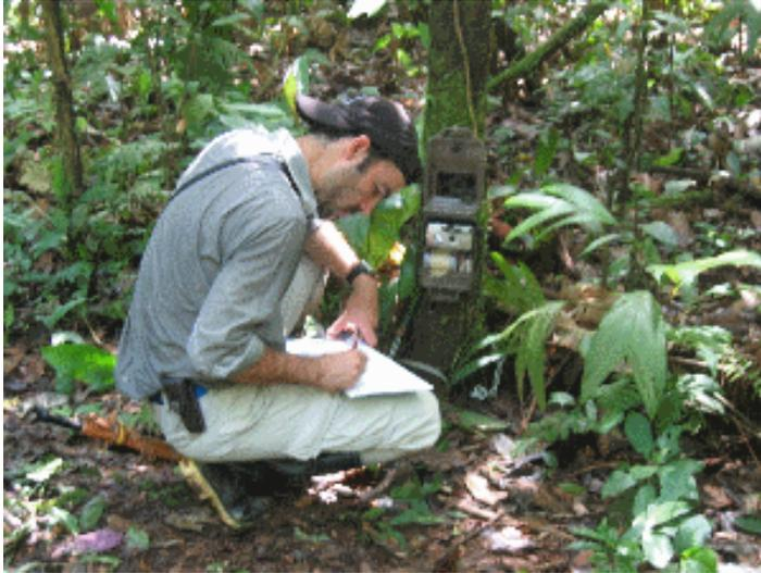
The PI changing film roll and batteries to one of the cameras. Camera traps operating in the Amazon, under extreme heat and humidity must be checked maximum every ten days to also replace saturated silica gel desiccant cushions and re-seal with silicone on the outside. This requires a significant logistical challenge in a 70 square km are with 20 camera stations. Picture by S. Durant.
