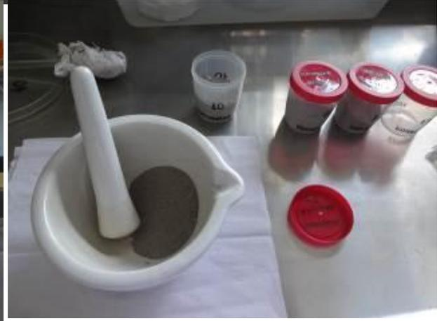
**Preparation of the sediment samples collected for organochlorine analysis.**
