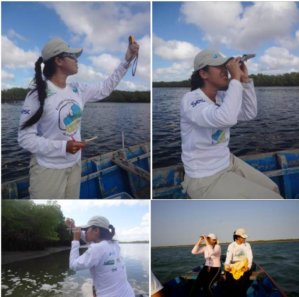
Measurement of wind speed and air temperature using anemometer and the salinity of water using refractometer.
