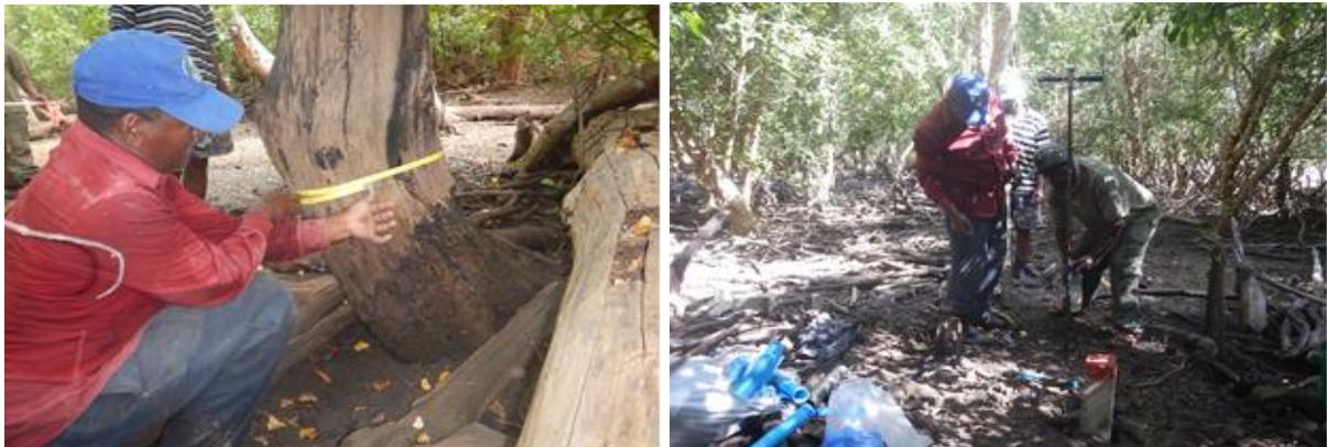
Field crew working at one of the plots in Wami Estuary. **Left:** Taking measuring of a standing stump. **Right:** Retrieving soil core using a Multi-stage sediment corer close to the plot centre (concrete mark with red paint at top).
