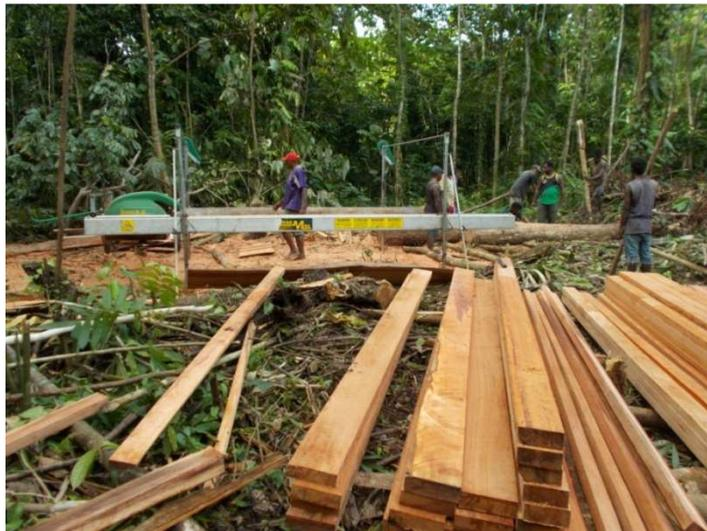
Figure 7: Milling of logs into precisely cut timber.
