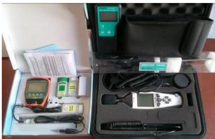
For microclimatic measurements in field conditions I bought next technical equipment: a) soil moisture meter Rixen M-700S (1 pcs.); b) soil pH and temperature meter Ezodo MP-103S (1 pcs.); c) environment multimeter Flus ET-965 (1 pcs.). This equipment will allow getting clear data about air temperature, air humidity, illumination, soil moisture, soil temperature, and soil pH in localities of investigated *Aconitum* taxa.
