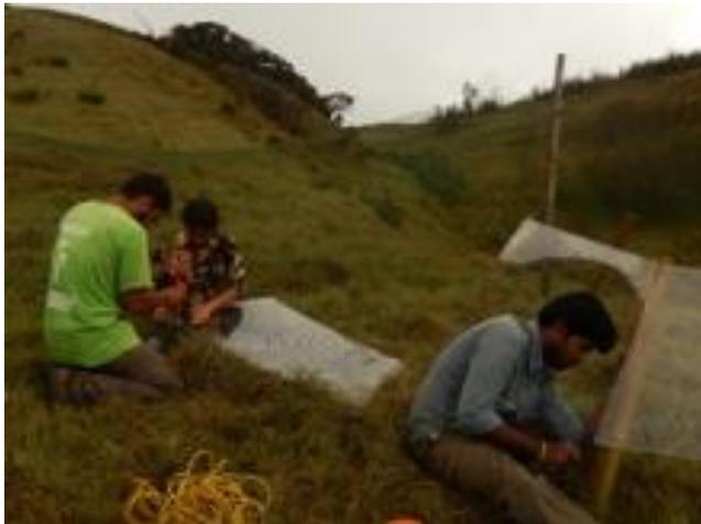
Picture 1: A number of warming experiments worldwide use open top chambers (OTCs) to study ecosystem responses to temperature rise. We modified the OTC design from Godfree *et al.* (2011), and after some setbacks, we have, we believe, OTCs that can withstand the high winds at our field site during the monsoon, despite the sloping terrain they are built on. The OTCs are hexagonal structures, ~3 m in diameter and ~50 cm tall. An iron frame supports the pyramidal structure made of
