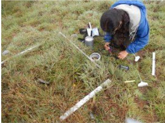
Picture 3: Vegetation cover and composition, soil chemistry, abiotic factors like soil moisture and temperature, and soil respiration are being monitored periodically. The photograph was taken while one of our team members was measuring soil moisture, soil temperature and soil respiration.
