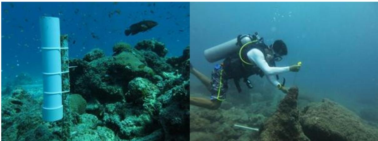
Left: A sediment trap deployed at one of the study sites. Right: Saw Darrick from DIVEIndia deploying a light data logger.
