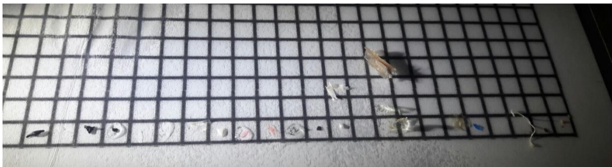
Figure 3. 5GYRES Manta trawl measurement grid used to categorize the size of the plastics found
