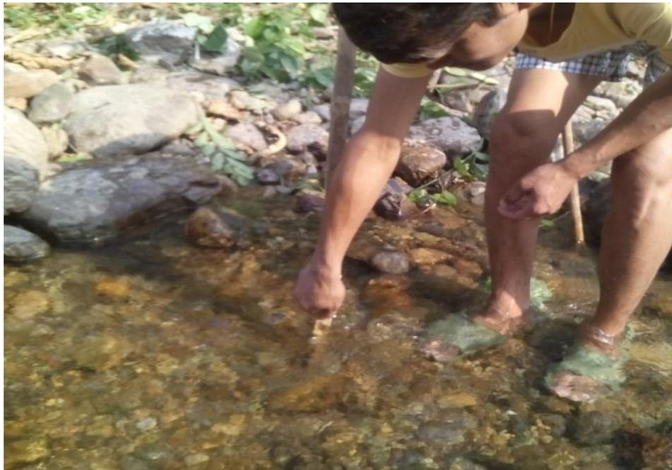
Figure 5. Stream gauging to find the volume of water discharge, Measuring the width and depth of stream at each 3.2 ft. respectively.
