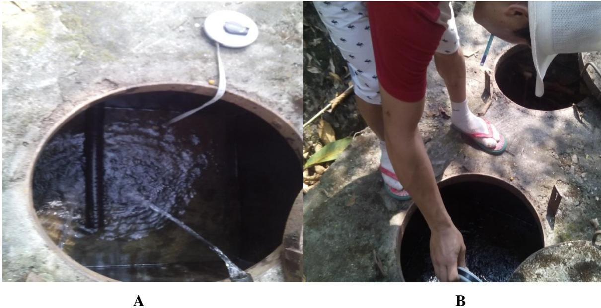
Figure 6. Volumetric analysis of drinking water. A: Measuring the new height in every minutes and B: Researcher measuring the height after 30 min.
