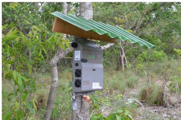
Audio recorders deployed on Barranco Alto farm, with associated temperature data loggers. The devices were placed at approximately 1.5 m above ground, in trees or wooden stakes, and always oriented toward the ponds. I also installed a small roof to protect the recorders from intense rain.
