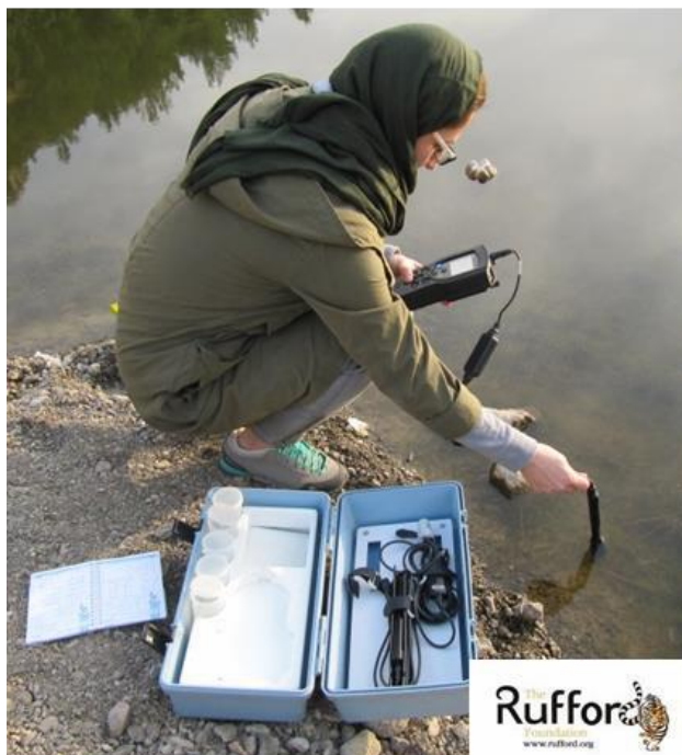
Measuring temperature, Dissolved Oxygen, pH, Salinity and Conductivity in the field
