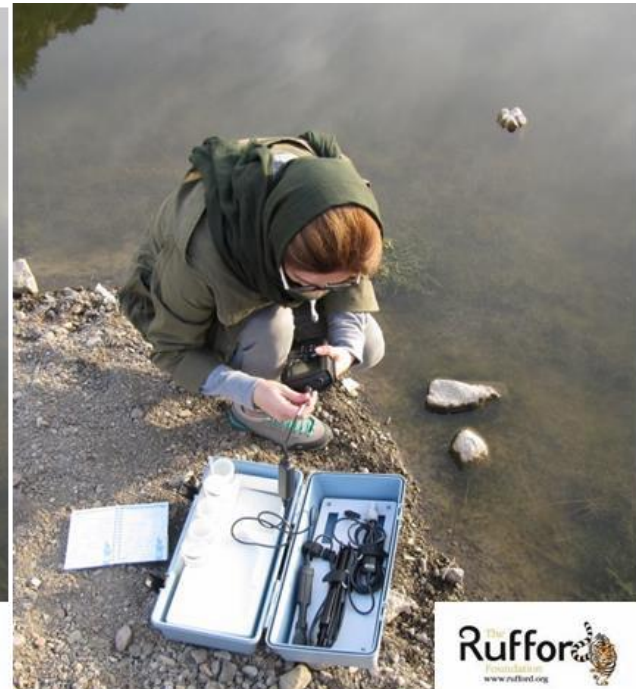
Measuring temperature, Dissolved Oxygen, pH, Salinity and Conductivity in the field
