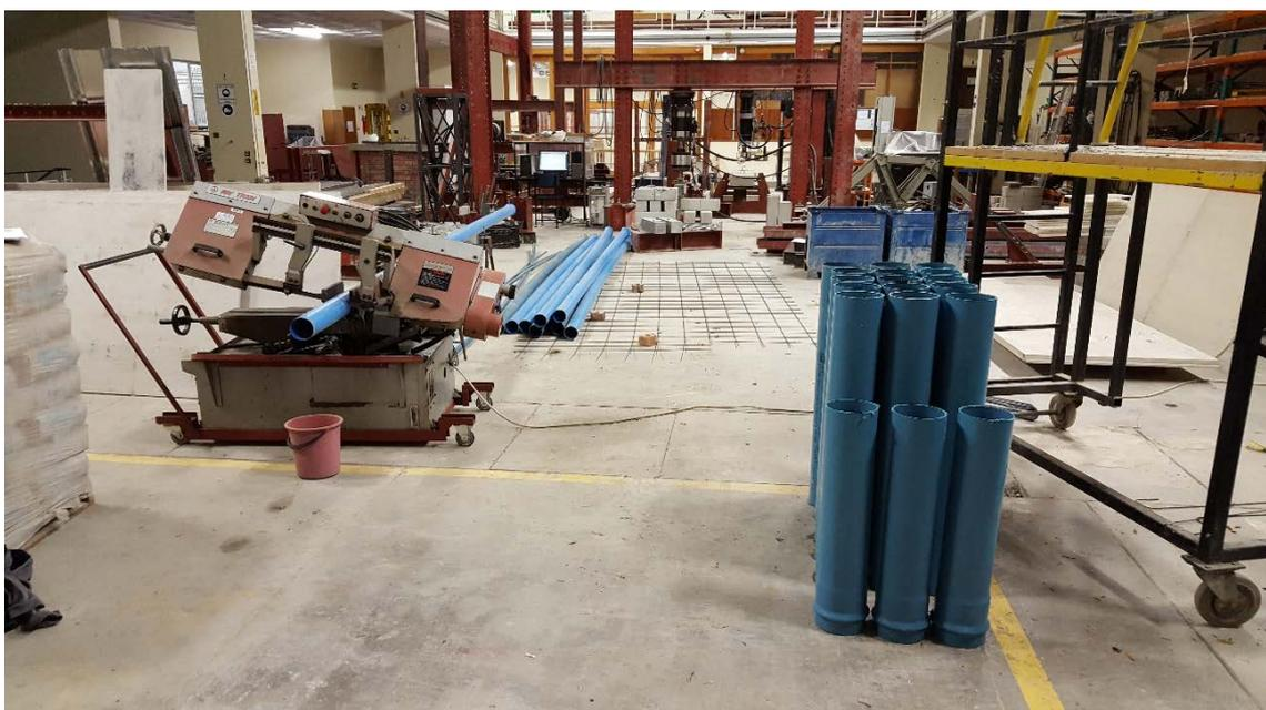
The materials needed for the water purification system are PVC pipes 110 mm and 160 mm diameter. The lengths needed were 60 m and 20 m for the 110 mm and 160 mm diameter pipes respectively. Using a table bandsaw the PVC pipes were cut into the correct lengths. It was established that the optimal depth of each silo is 500 mm, to allow for plant growth, water permeability and a gravel and sand filter with the chamber, above the drainage pipe.
