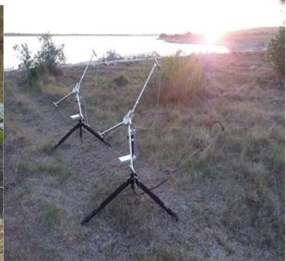
Left: Ultrasound gate receiver connected to laptop. Right: Set up of multiple microphone arrays to record echolocation calls of free flying bats in a foraging site in Fynbos biome at Dehoop Nature Reserve.
