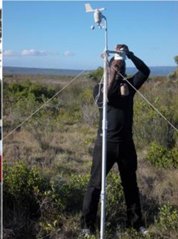
Left: Set up of multiple microphone arrays to record echolocation calls of free flying bats in a foraging site in Fynbos biome at Dehoop Nature Reserve. Right: A portable weather station to record weather parameters (temperature, relative humidity, atmospheric pressure and wind speed) at the same while recording echolocation calls.
