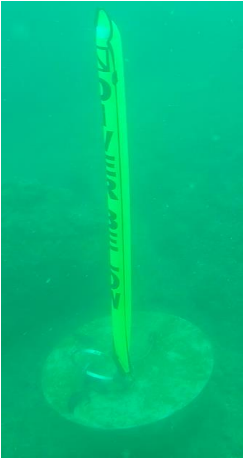
Fig 1. Underwater anchor site at Morro Mico for one of the Ecological Acoustic Recorders (EARs) from Oceanwide Science Institute. The EAR has been removed in this image but attachments and a bright buoy for searching ease have been left for next year's deployment.
