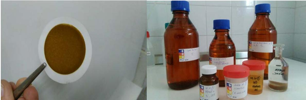
Left: Filtered water sample for chlorophyll a and cyanotoxin analysis. Right: Samples in the laboratory.
