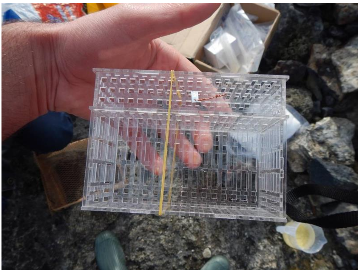
Fig. 4 Whitlock-Vibert Box used in experiments
