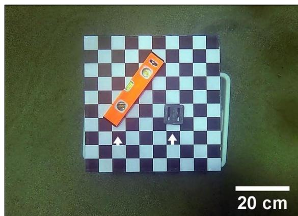
**Figure 5:** Grid of 50cm and two laser dots pointed by the white arrow for calibration.
