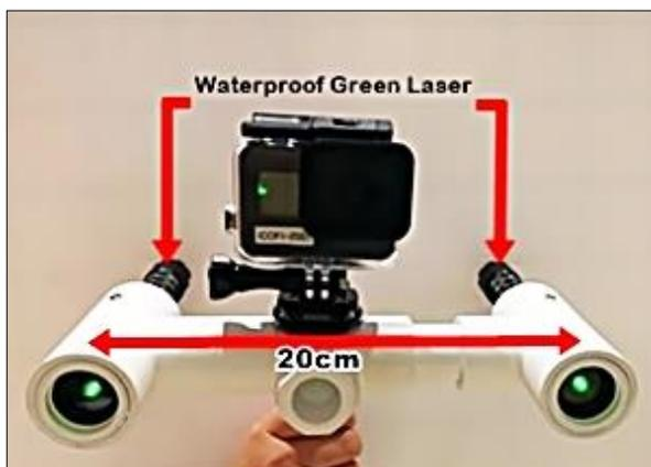
**Figure 4:** The laser units with 20cm apart and Go Pro camera.
