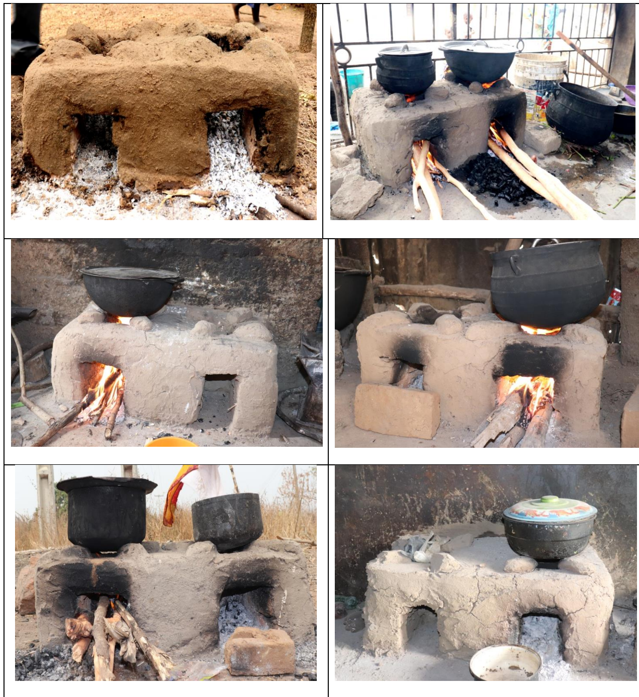
Two-phase Improved and Efficient Biomass Cookstove in use by households
