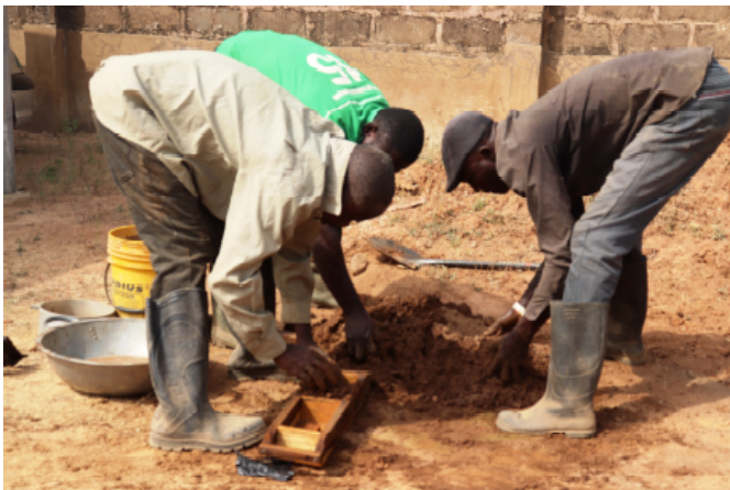
Left: Hand mixing of clay, topsoil, manure, sharp sand and water, then putting of the mixture in mould to make clay blocks (© Fola Babalola). Right: removing of the clay blocks from the mould and assembling of the blocks to dry in sun (©Fola Babalola) .
