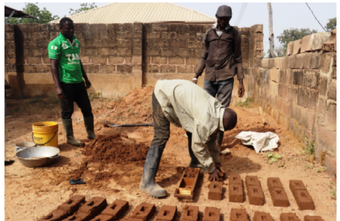
Left: Hand mixing of clay, topsoil, manure, sharp sand and water, then putting of the mixture in mould to make clay blocks (© Fola Babalola). Right: removing of the clay blocks from the mould and assembling of the blocks to dry in sun (©Fola Babalola) .
