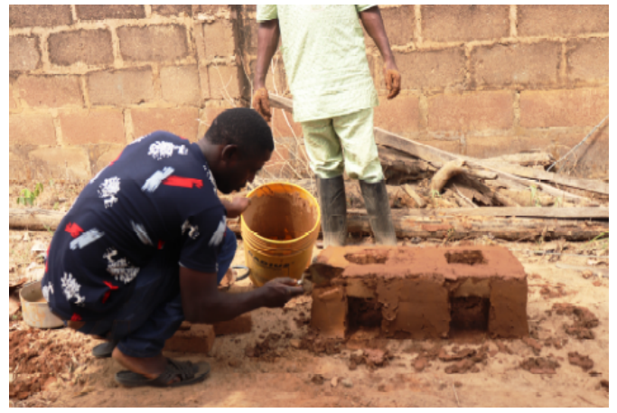
Left: Assembling of clay blocks to make the biomass efficient cookstove (© Fola Babalola). Right: Making prototype of the biomass efficient cookstove (© Fola Babalola).
