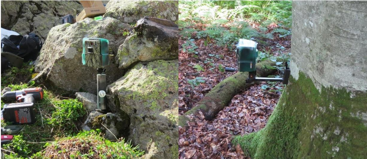
**PHOTO 16; 7: CAMERA TRAPS IN WORKING CONDITIONS, ON HAND-MADE (LEFT) AND HME (RIGHT) MOUNTS.**
