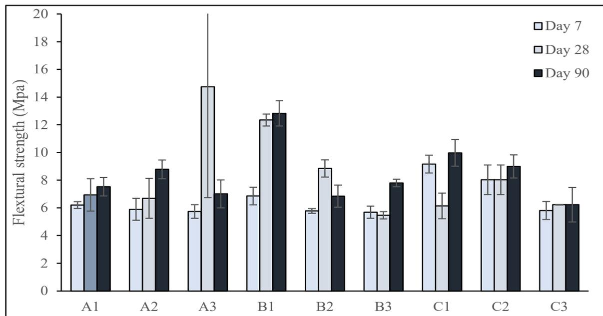
Fig. 4. Flexural strength of different mix designations on day 7, 28 and 90 (%).
