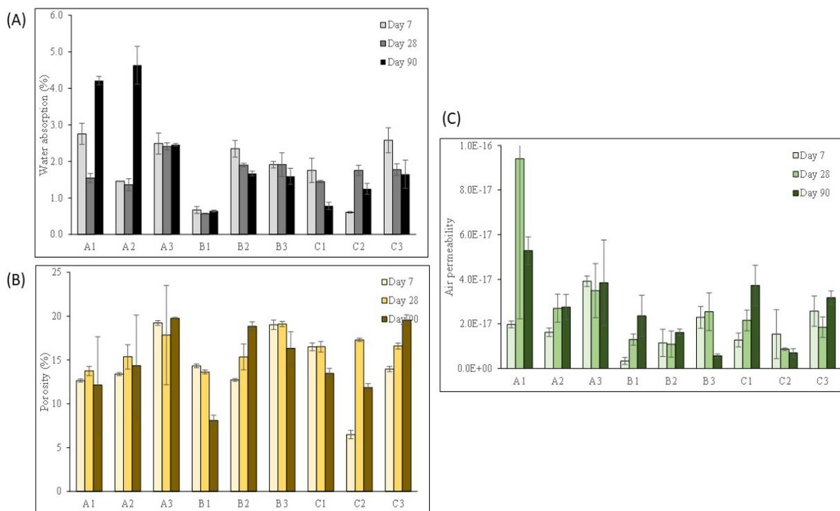
Fig. 5. Tests conducted in 7 days, 28 days and 90 days on the different mix designations (%): (A) Water permeability, (B) Porosity, and (C) Air permeability.
