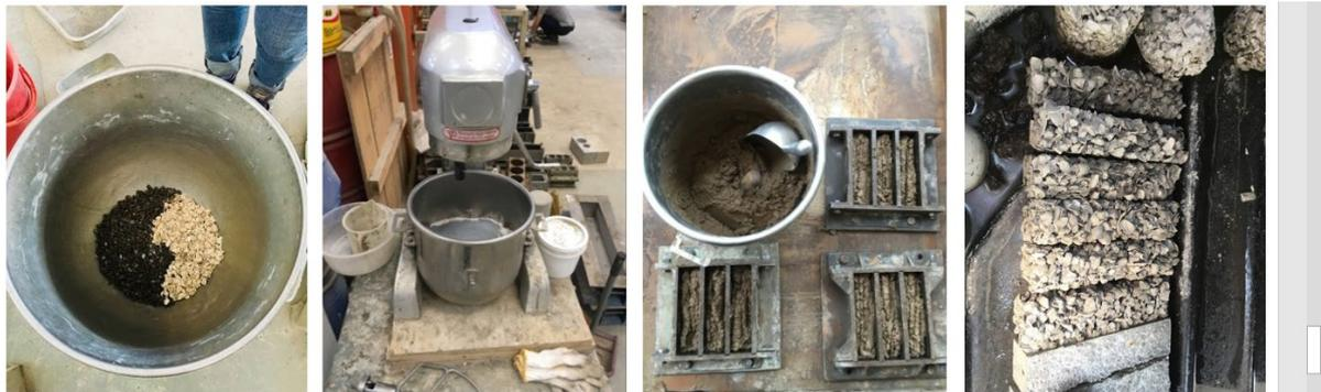
Fig. 1. Eco-concrete produced with quarry dust and crushed shells as coarse aggregate.
