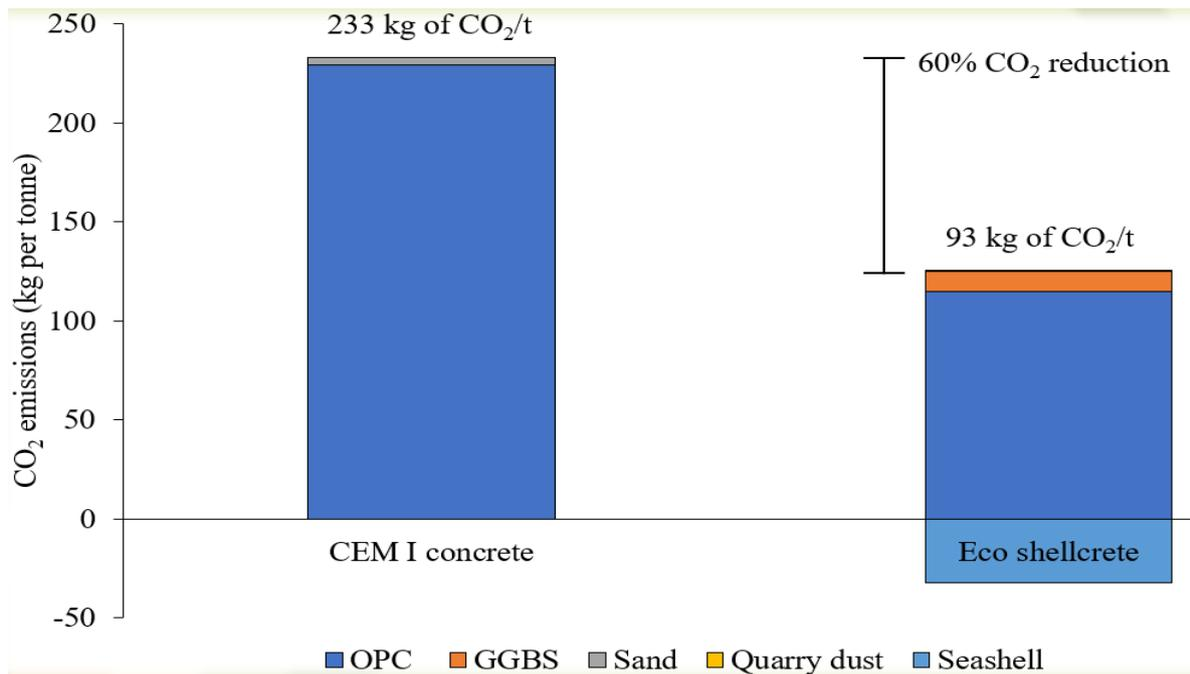
Fig. 2. Carbon dioxide emissions of Portland cement concrete and eco-concrete. CEM I concrete = Portland cement concrete.
