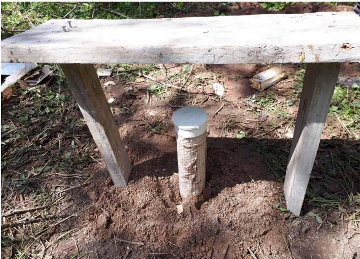
Photo 2. A freatimeter installed inside the forest.
