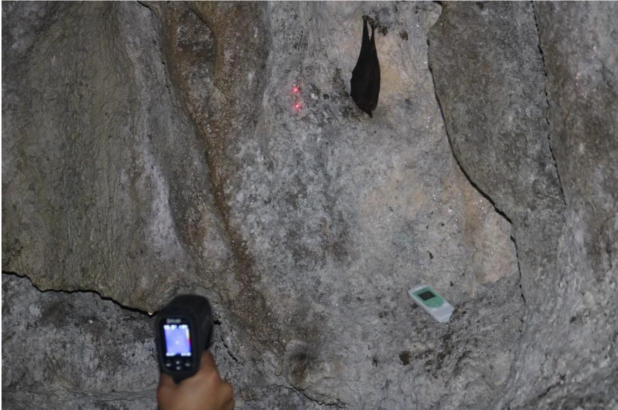
Picture 3- A tempnote is placed near the roosting location of *Rhinolophus luctus*. The difference in cave wall temperature and that of bat is taken using a TG-165 thermal camera.
