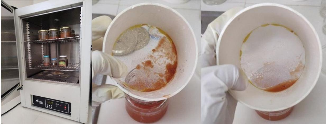
Figure 1: Samples in the organic matter digestion process. Figure 2. Sample filtering through two different meshes.
