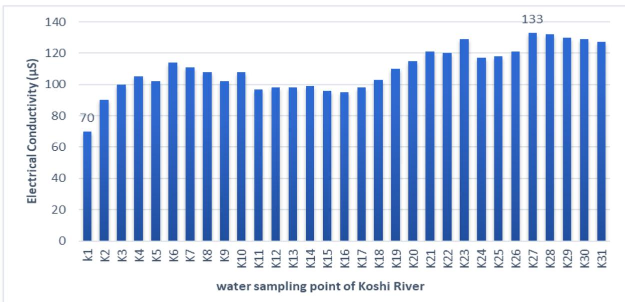
Figure 4: Electric conductivity at different sampling points of Rivers
