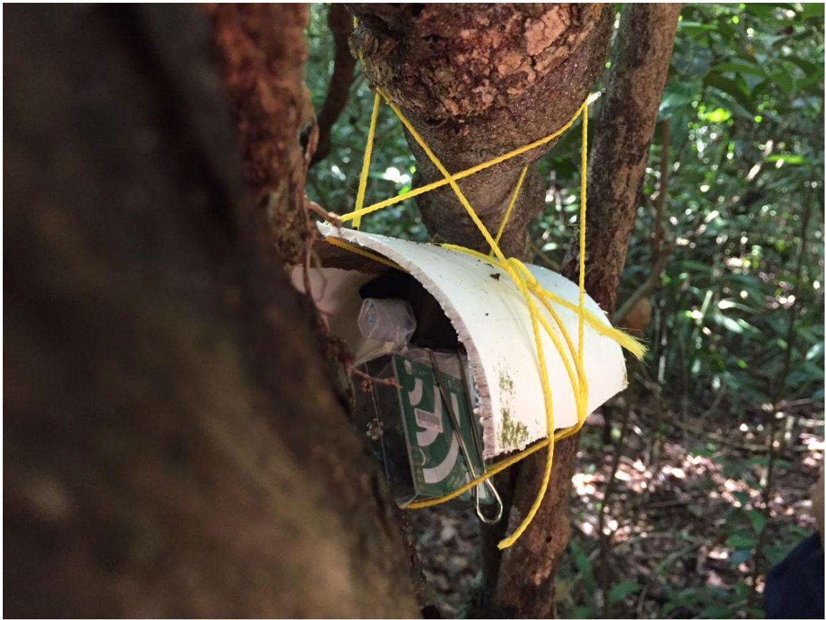
Photo 2: Testing how our Audiomoth recorders can be protected from rain using little roofs made of recycled PVC pipes. Photo 3: All work was carried out following the principles of “Best Practices in Field Primatology in the Age of COVID-19”. Among others, team members were tested for COVID-19 before starting field work.
