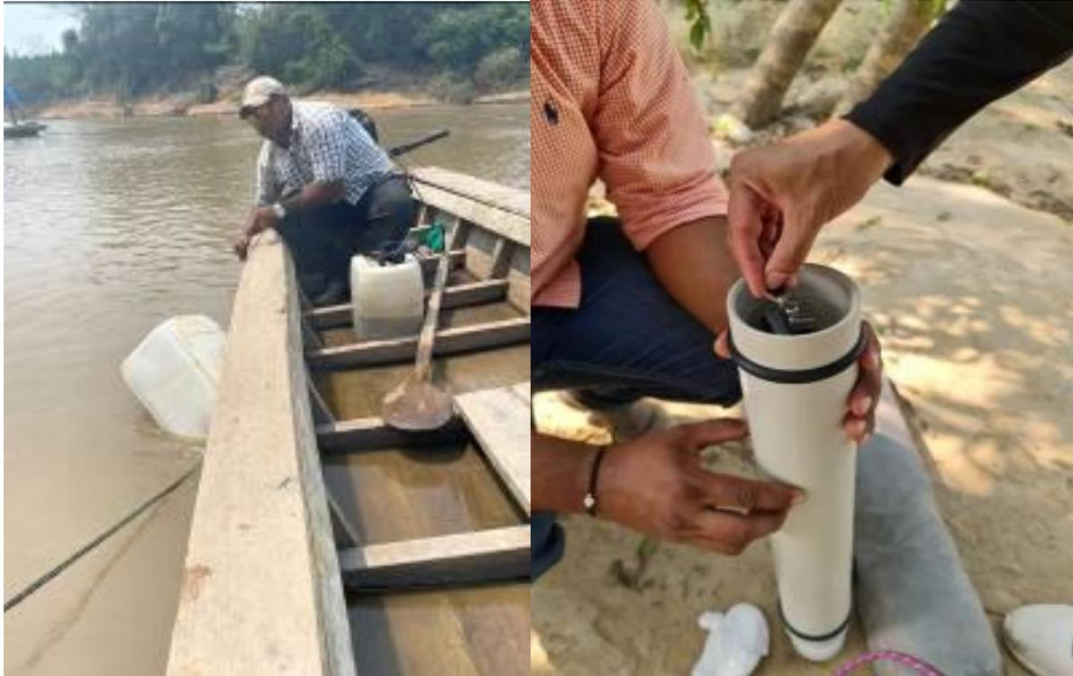
**Figure 2.** I work with the F-POD, involving the installation and periodic inspection of the equipment. This device has been in place for almost a year, continuously recording information in the Pojije River, Beni, Bolivia.
