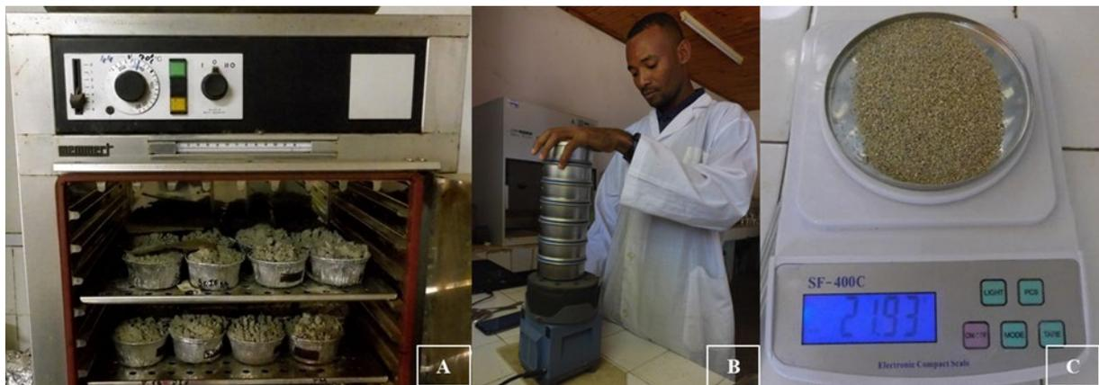
Photo 3: Photo showing the stages of sediment sample analysis in the laboratory: A) drying in an oven, B) sieving with a shaker and C) weighing the rejects after sieving
