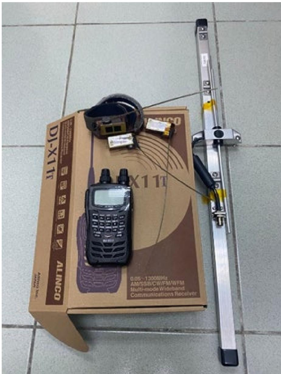
Figure 5: Three satellite transmitters, Allinco Receiver and Yagi antenna bought for satellite tracking.
