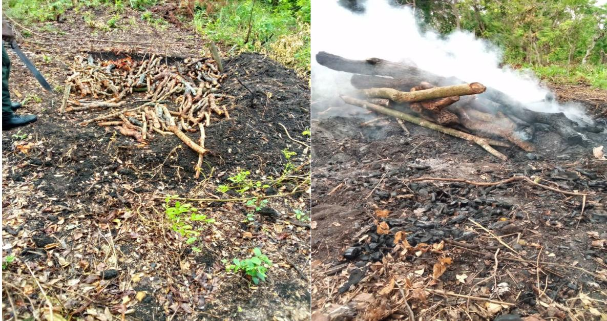
**Figure 9.** Charcoal kiln construction. **Figure 10.** A fresh charcoal kiln.
