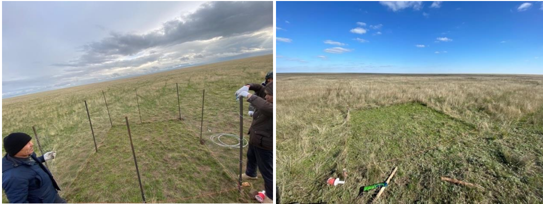
Figure 2. Examples of fenced and open biomass assessment plots. Poles for the fences were buried at a depth of 50 to 70 cm. Photo: Aibat Muzbay.
