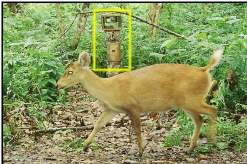
*Camera and the sensor unit mounted on wood, while a hog deer being photographed from the opposite end.*
