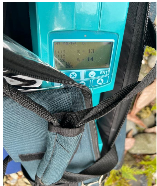
In situ measurement of atmospheric mercury using a portable analyzer (Lumex), reporting gaseous mercury concentration ( \text{ng m}^{-3} ) at the study area.
