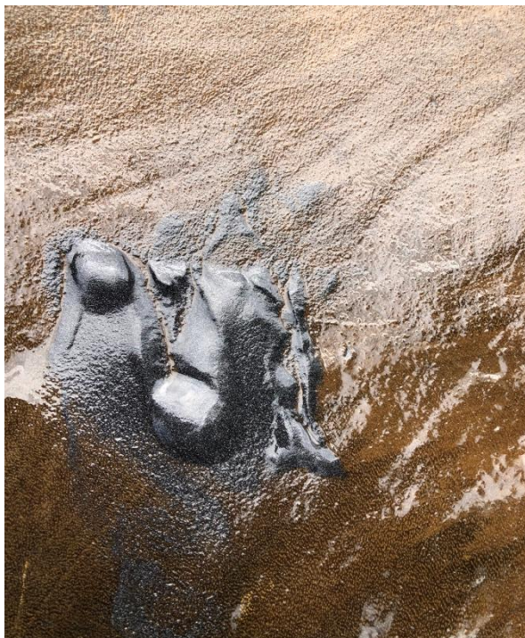
Visible mercury contamination in soil at the sampling site, showing metallic mercury droplets accumulated on the wet surface.
