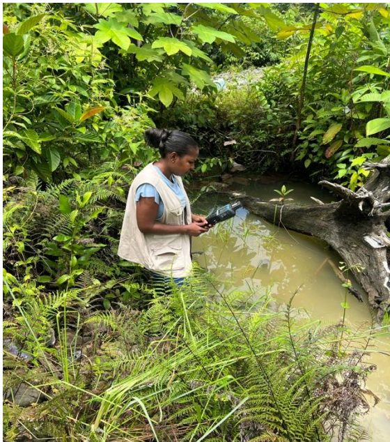
In situ measurement of water physicochemical parameters in a mining pond using a portable multiparameter instrument. Photographer: Juan David
