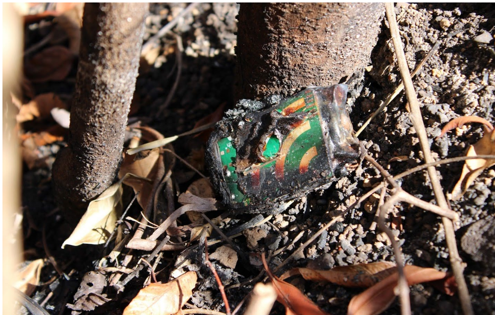
Figure 2. An acoustic recorder damaged by the fire.
