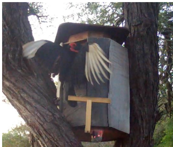
Figure 3. A ground-hornbill at an artificial nesting site with the prototype perch scale fitted to it.
