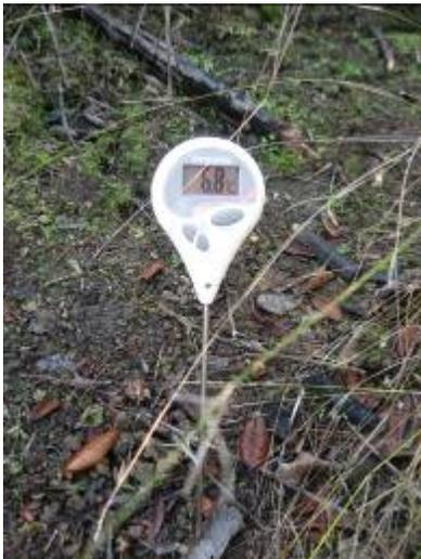
**Image 11.** Soil thermometer (measurement range: -10 to 200°C).
