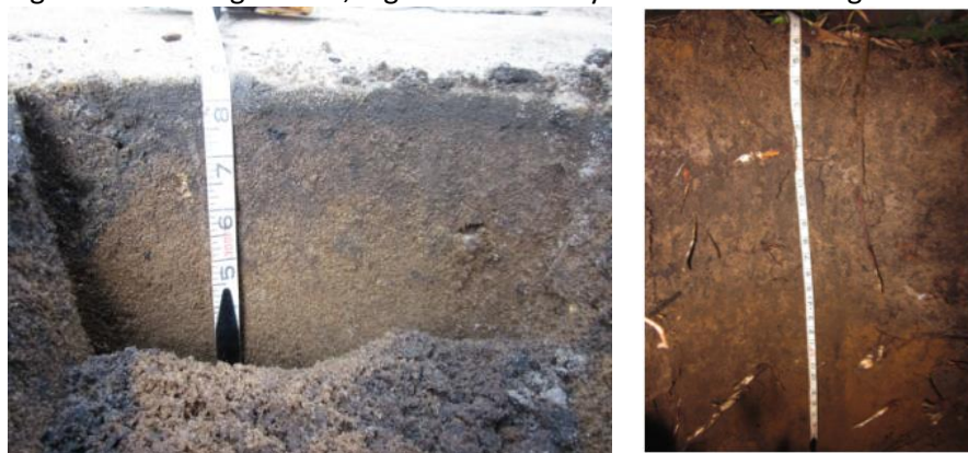
Figure 1. Left: original soil; Right: soil after 5 years of conditioning
