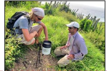
IRF staff geologist **Dr. Carlos Ramos-Scharrón** (right) describes the uses of an automated rain gauge in erosion studies to a volunteer. Rain provides the energy and the medium for erosion and sediment transport and is used to predict erosion rates from natural hillslopes and from ground that has been disturbed by construction, unpaved roads and foot trails, and agriculture.
