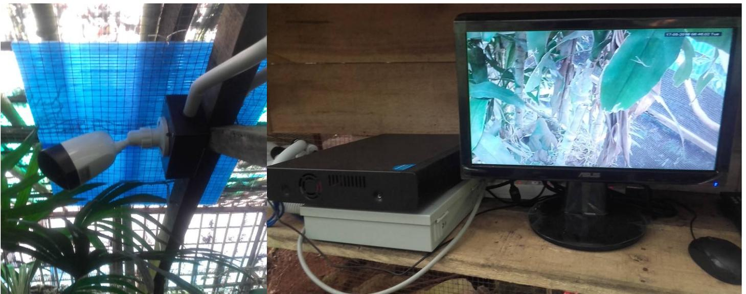
**Picture 4.** CCTV system installed in one of our buildings: High-resolution camera with cables protected into safe box and PVC pipes (left). Screen and electrical installation protected against lightning (right)
