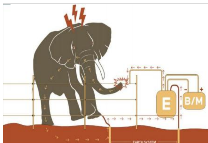
Figure 3. Schematic diagram illustrating how the electric fence operates. Source: Space for Giants, 2023.
