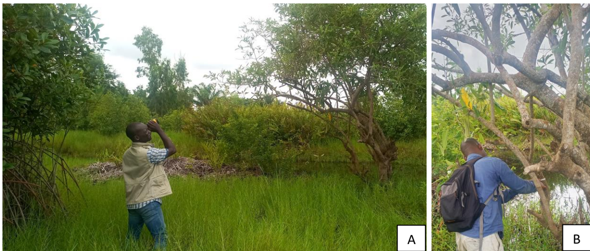
Photo 1: (A) total height (H; m) measurement using a digital hypsometer (Nikon Forestry Pro II Laser) and (B) diameter at breast height (DBH) of mangrove (tree measurement on the field).
