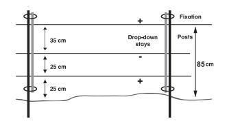
**Fig. 2.** Design proposal of a guanaco friendly high tensile electric fence for livestock in arid Patagonia. Hot and ground wires are attached to drop-down stays that are fixed to posts. Top wire height is lower than current ovine design and larger space between wires would allow crossing of yearling and reduce entanglement.
