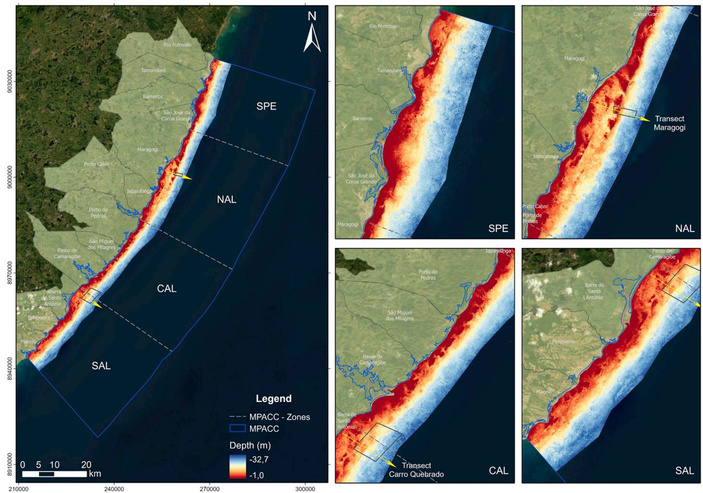
Fig. 5. Spatial variations of shallow bathymetry models created using 24-month mosaics. Zoom of the four sectors of the marine protection area. The bathymetry represents the spatial variation of the benthic geomorphology. Sector ID as in Fig. 1.
