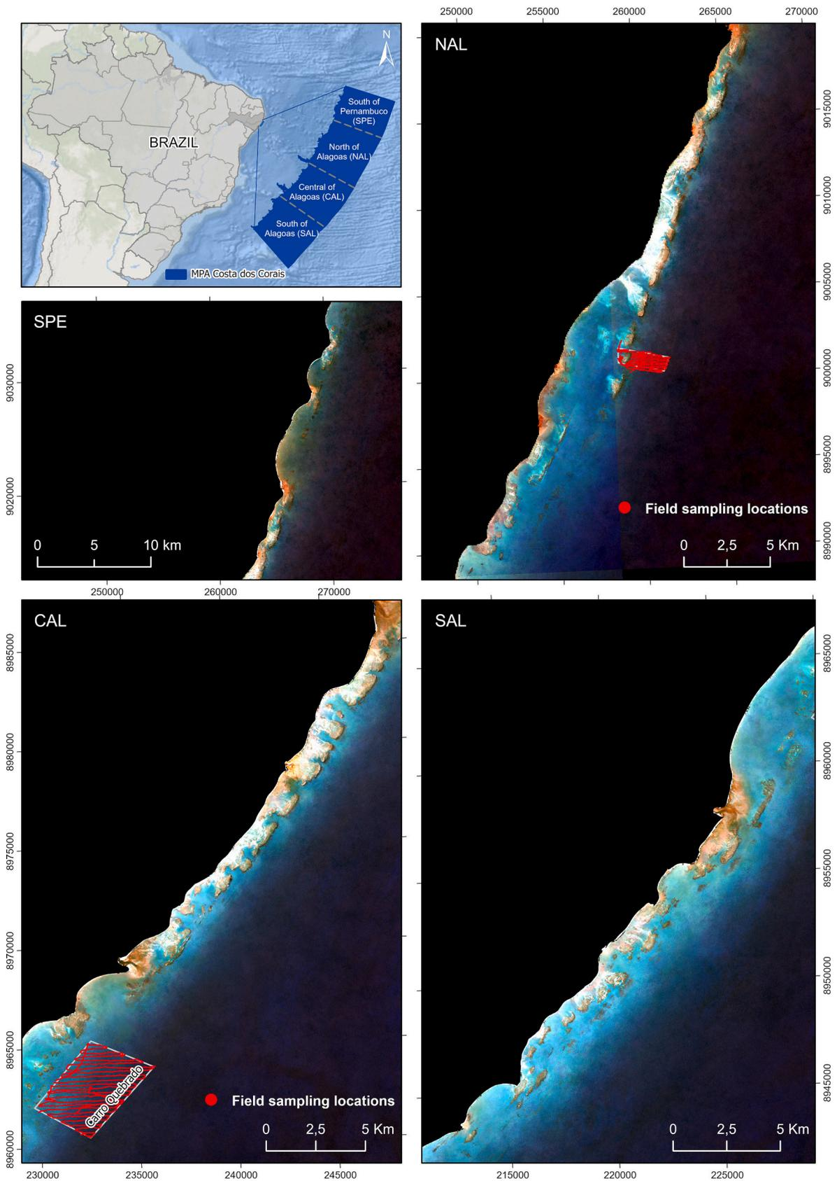
**Fig. 1.** Study area for bathymetric and geomorphological mapping. Sentinel-2 true color mosaics (24-month mosaic) and field sample locations Maragogi (15.481 points collected) and Carro Quebrado (18.427 points collected). Yellow pixels are no-data areas, mostly located in surf zones or areas above sea level. (For interpretation of the references to color in this figure legend, the reader is referred to the web version of this article.)
