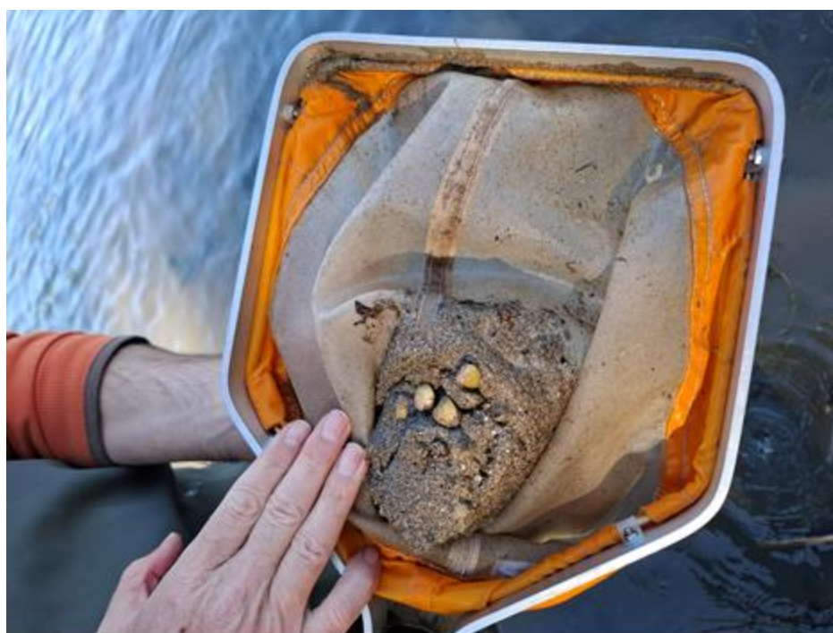
Photo 31: Sampling, bentho-sampler net (25x25 cm, 500 \mu m mesh size)
