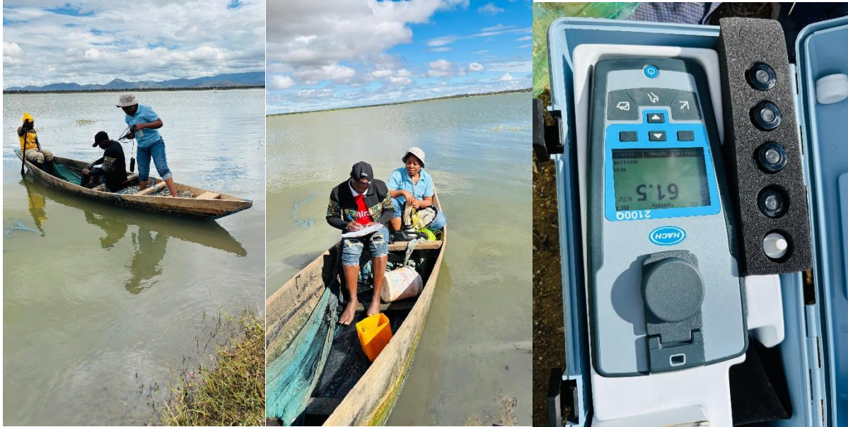
Figure 02: Measuring dam's water quality including the dissolved nutrients, pH, water temperature, dissolved oxygen, turbidity and salinity at Hombolo Dam-Dodoma. Photo credit © Rosemary-UDOM 2025.
