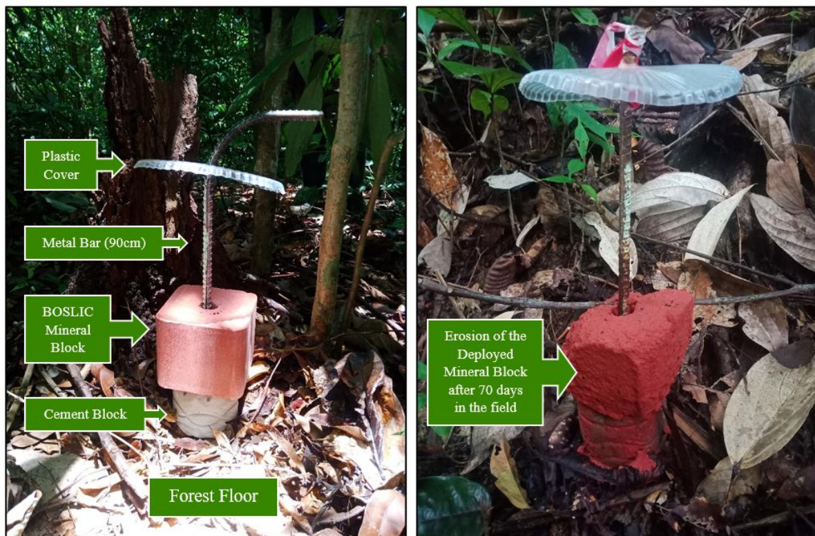
Picture 1. Design of the artificial saltlicks established at half of the sampling points
